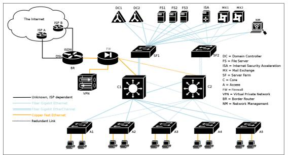
The internal network is protected by a Cisco PIX for security.
